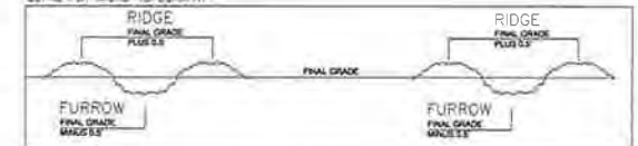
FLOW ON CONTOUR WITH MOLDBOARD PLOW
