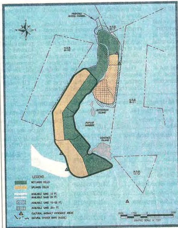
The current recommended alignment for the Poplar Island Expansion study indicates a large addition to the North of the island. The area outlined in black signifies the island's current shoreline.
