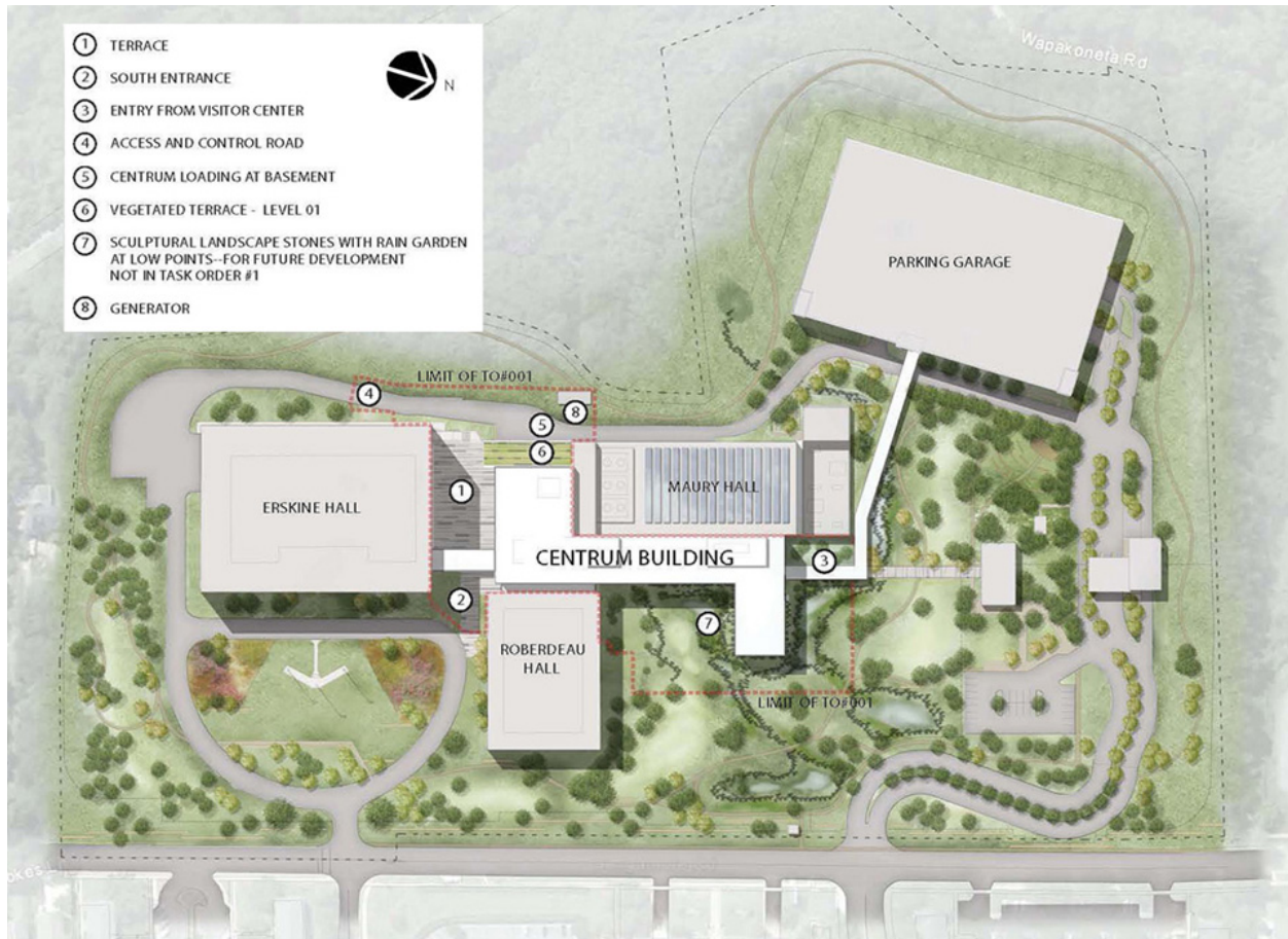
Figure 3: Site plan of Centrum with the project's limit of disturbance (Image date: June 6, 2013)
