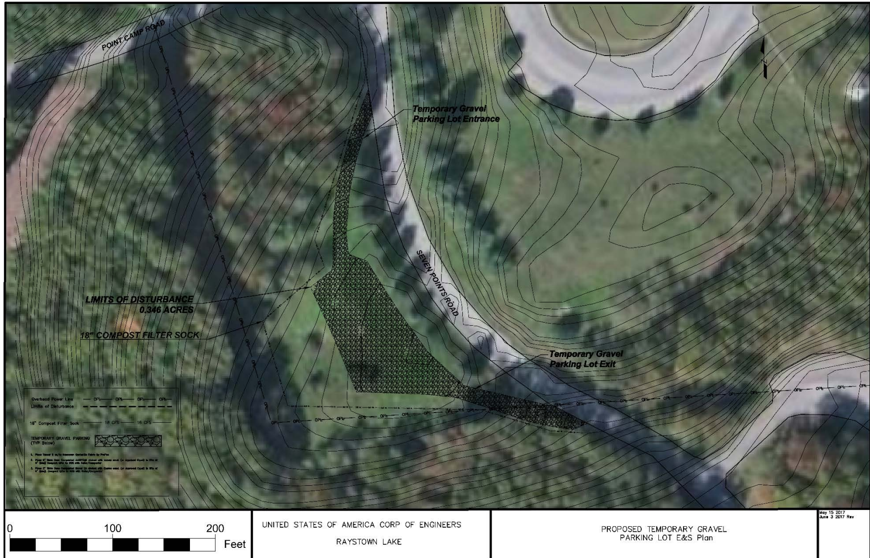
Figure 2. Temporary Parking Lot Site Plan
