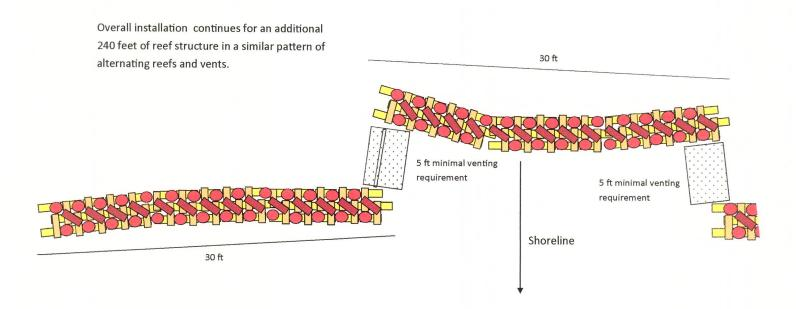
An example of installed reef sections is depicted. The installation will be set just below the MLW line. The proposed reef sections will be placed approx. 20-25 feet from MHW.
