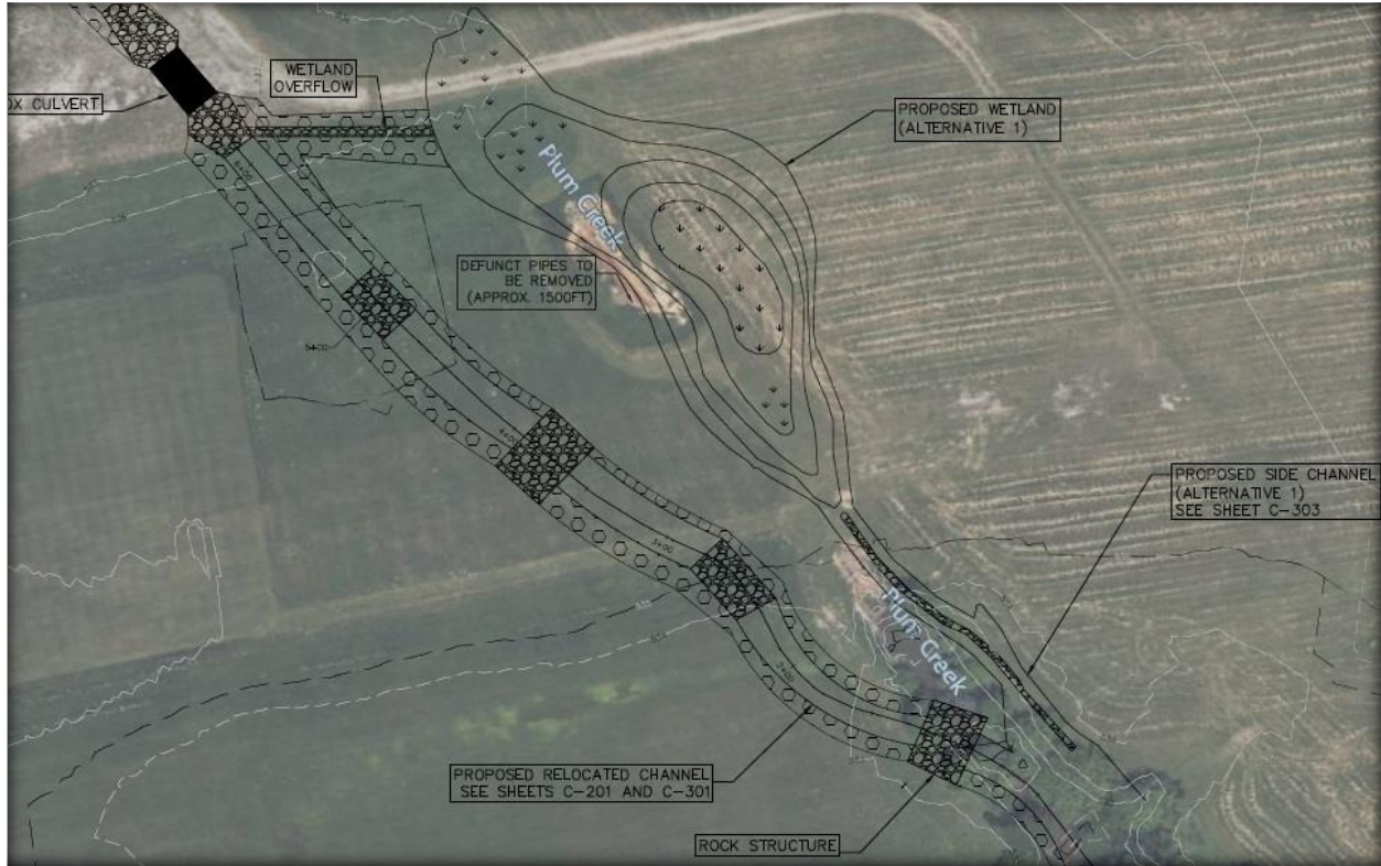
Figure 7, showing side channel and overflow channel, including a portion of relocated channel.
