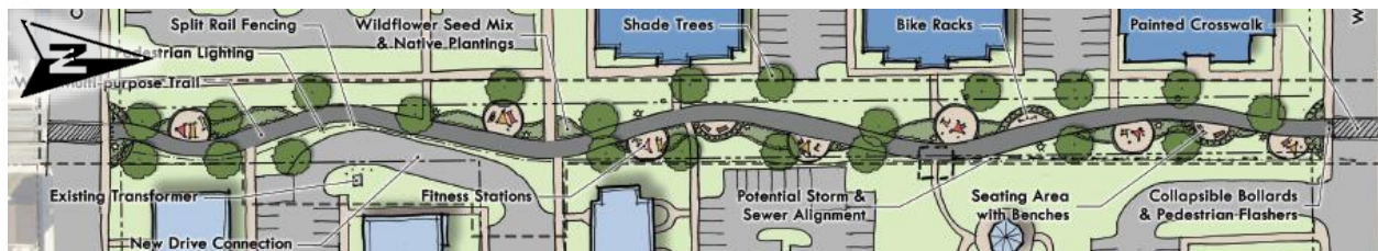
Visual 3.15-3: Chambersburg Rail Trail Linear Park – S Water St between W Catherine St and W Washington St (conceptual)
