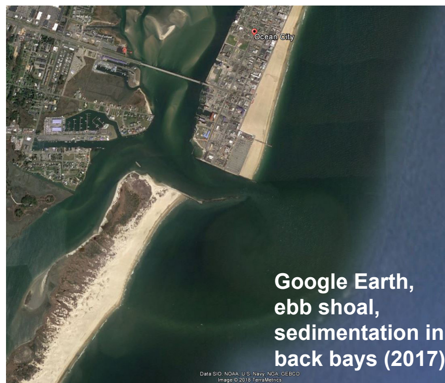
Ebb shoal, sedimentation in Sinepuxent and Isle of Wight Bays (2005)
