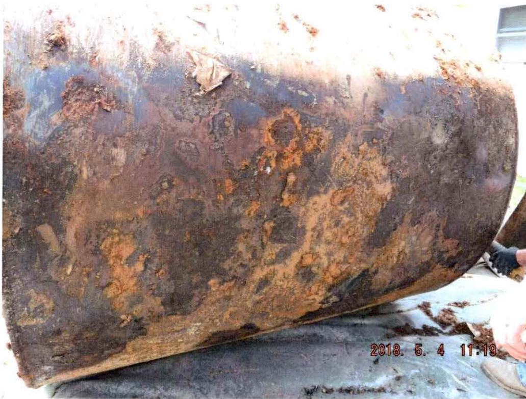
Figure 2 Bottom of the tank where the small hole was.
