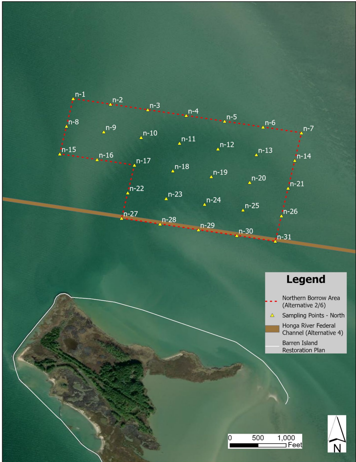
Figure 6. Boring Locations Investigated in the Second Geotechnical Investigation of the Northern Borrow Area
