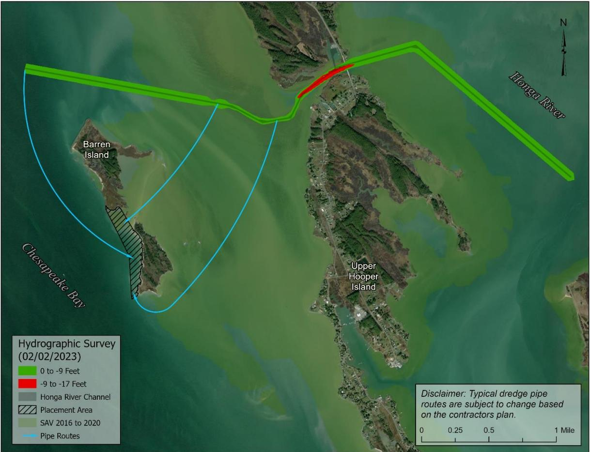
**Figure 2. Water depths in the Honga River Channel and Approximate Pipeline Locations.**
