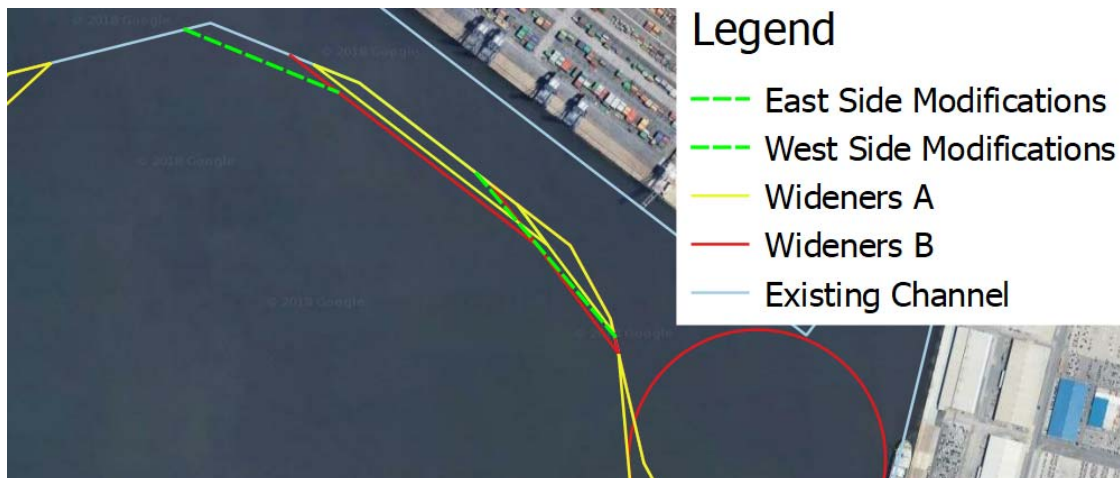
Figure 5-2: Channel modifications (dotted green lines) in addition to the Widener A and B designs
