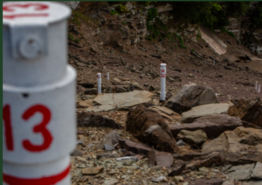
CLOCKWISE FROM TOP: A cable and sensor device sits on the ground near a marked pipe - a piezometer - along the side of Alvin R. Bush Dam. ■ A smaller tube inside the marked pipes drops down to a specific depth in order for engineers to measure pressure within the earth and rockfill dam. ■ Raj Singh, an engineer with the Baltimore District Geotechnical Branch lowers a sensor and cable into piezometer number 10. ■ Singh checks the measurement on the cable after being alerted by the sensor and pulling it back to the surface. ■ There are numerous marked piezometers that allow pressure to be regularly monitored at various depths and locations. ■ A view of the bridge to Alvin R. Bush Dam. ■ Engineers with the USACE, Baltimore District, Geotechnical Branch conduct inspections at Alvin R. Bush Dam. ■ The view downstream from the crest of the embankment at Alvin R. Bush Dam, located approximately 8.4 miles above the mouth of Kettle Creek and about 15 miles above Renovo, Pennsylvania, Aug. 18, 2020. (U.S. Army photos by Christopher Fincham)
