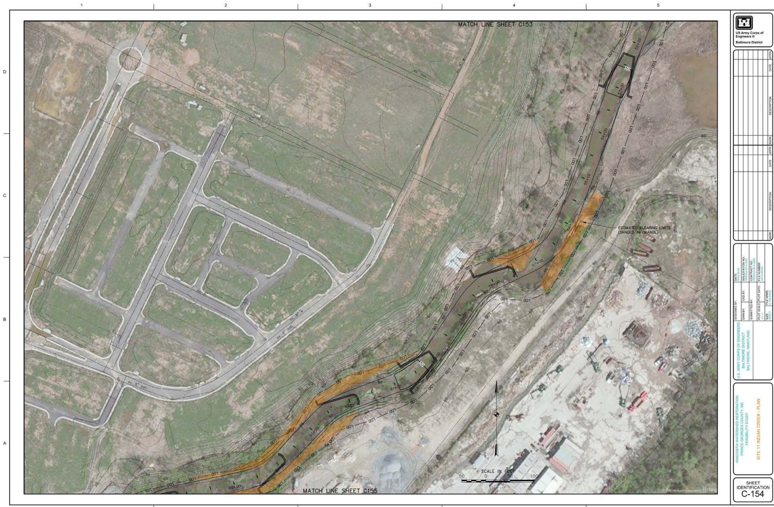
Figure 4-4. Design Sheet #154 - An example of structures, contouring, and clearing for Site 11 on Indian Creek.
