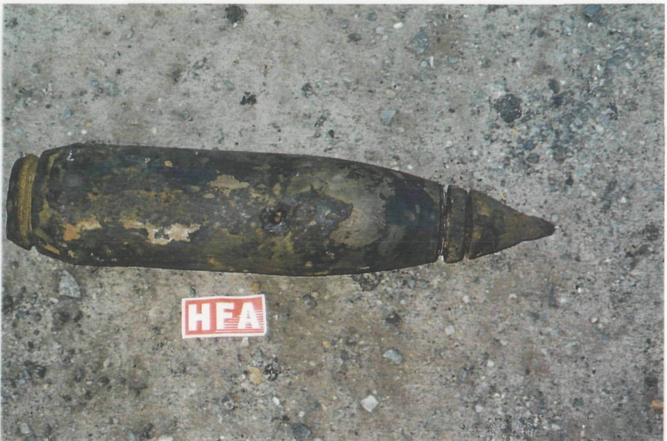
This 5 inch warhead has been shot with a jet perforator, note the small hole. The explosion also knocks all the rust and debris from the round also.
