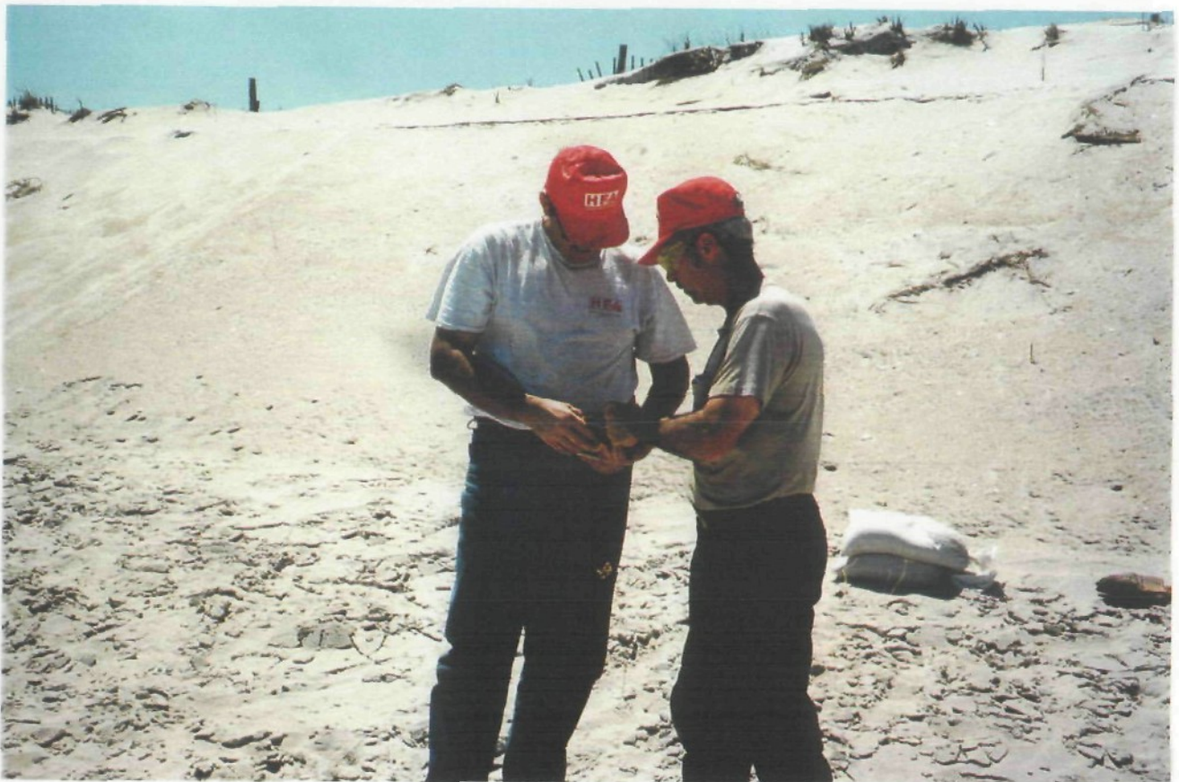
These two UXO Specialist are using a galvanometer to check the bridge wire of the blasting cap to ensure it is intact and has the correct resistance to explode the explosive when it charged with electricity.
