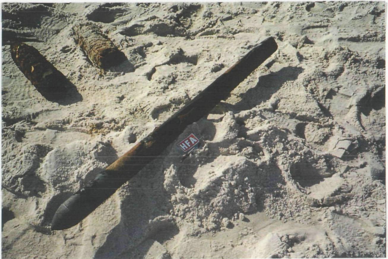
In the foreground is a 2.25 inch rocket. The two items to the rear are 5 inch warheads. These warheads are fitted to a 3.5 in rocket motor, not shown in the picture.
