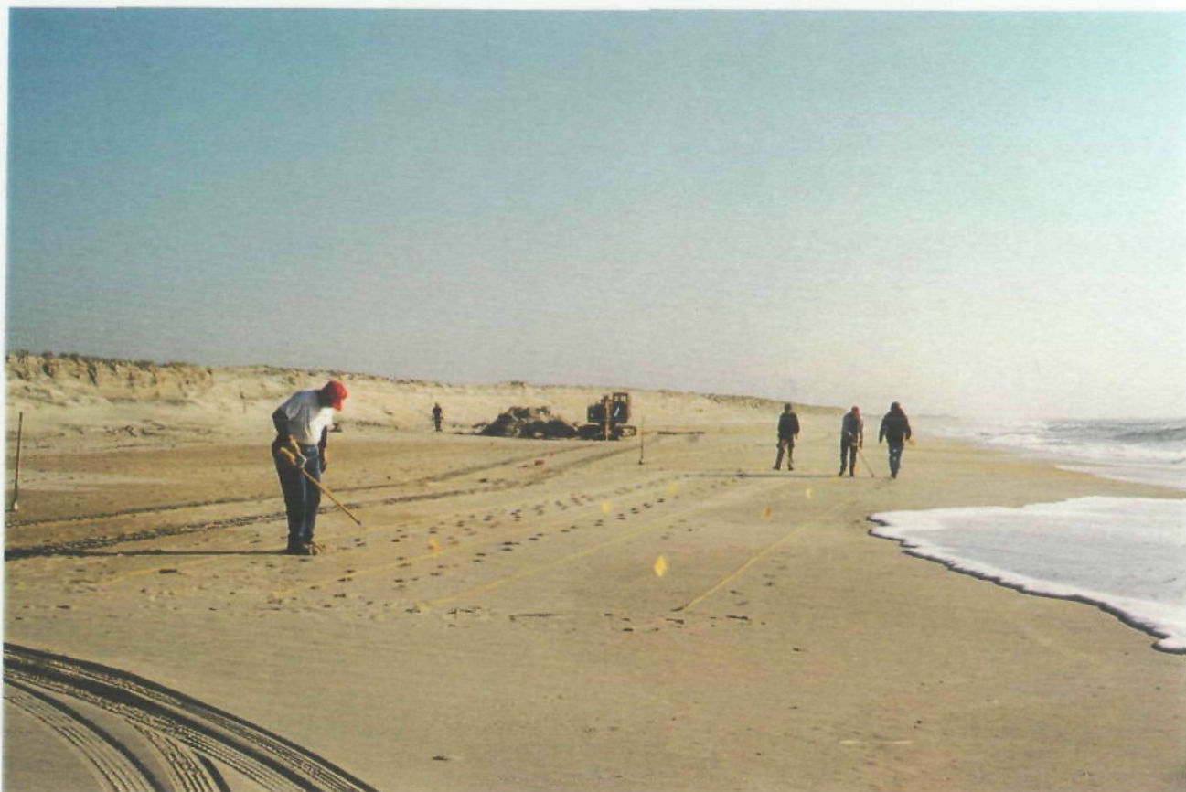
Each lane is then thoroughly search with a magnetometer. If a magnetic anomaly is located, it is marked with a yellow flag.
