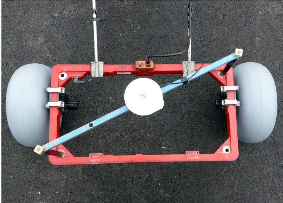
FIGURE 1-7 GPS ANTENNA POSITION ON HAND-PULLED ENCASED COIL
