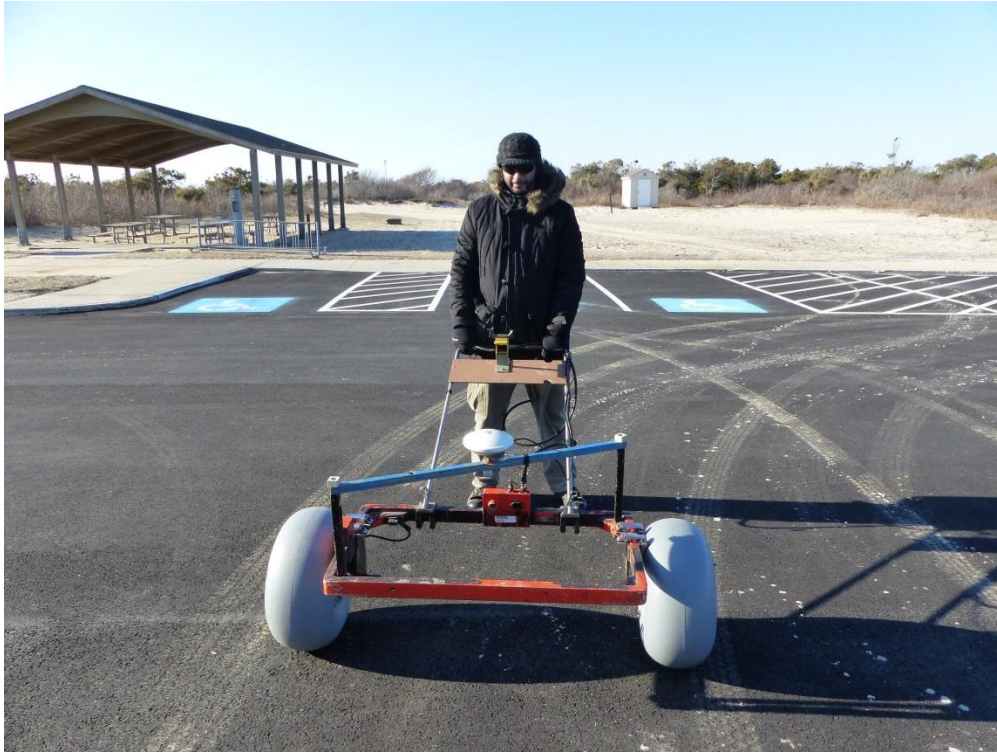
FIGURE 1-3 HAND-PULLED CART WITH BALLOON TIRES AND STANDARD EM61 Mk2 COIL
