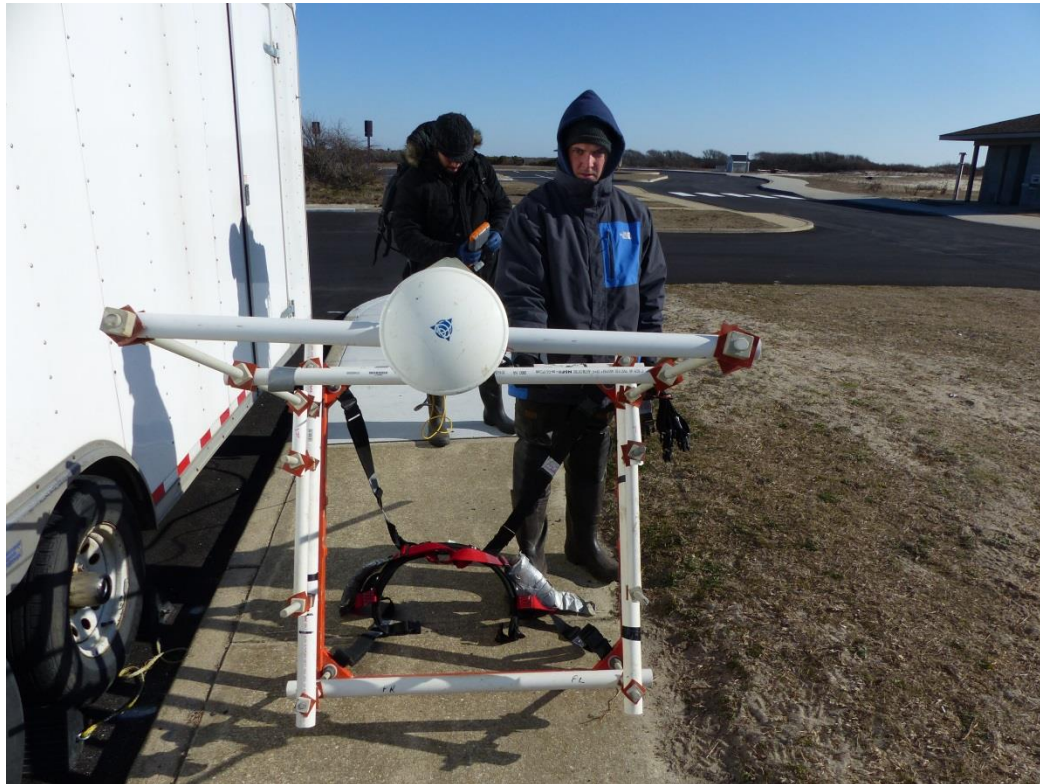
FIGURE 1-10 GPS ANTENNA POSITION ON SKIRT MODE 1 x 1 METER COIL
