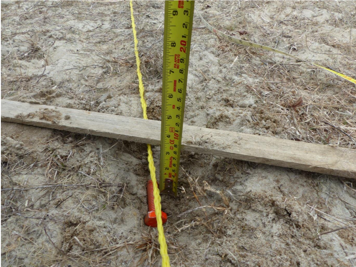
IVS-1: 5/8 inch-11 by 2" Bolt, Inline, Depth to center mass 3 inches.
