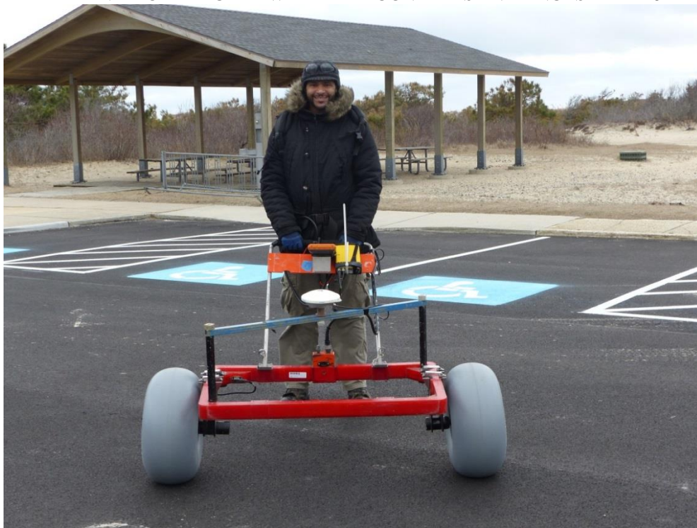
FIGURE 1-2 HAND-PULLED CART WITH BALLOON TIRES AND ENCASED EM61Mk2 COIL
