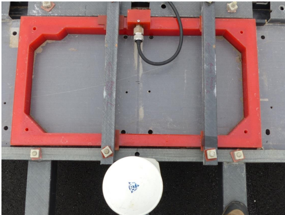
FIGURE 1-6 GPS ANTENNA POSITION ON TOWED SINGLE MARINE COIL
