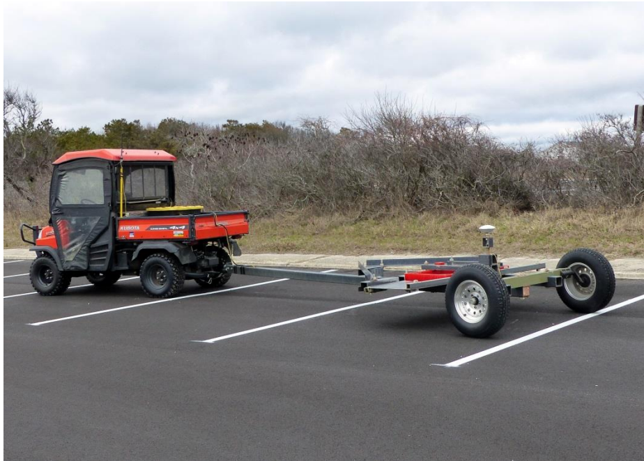
FIGURE 1-1 VEHICLE TOWED 0.5 X1.0 METER EM61S MARINE COIL
