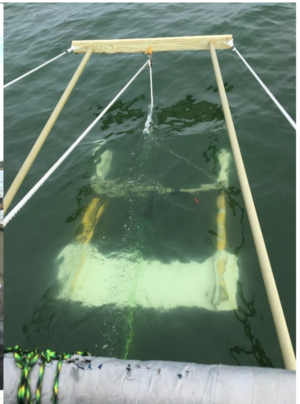
MRS 01/03 – Shallow Water DGM system on boat and in water set for collecting data
