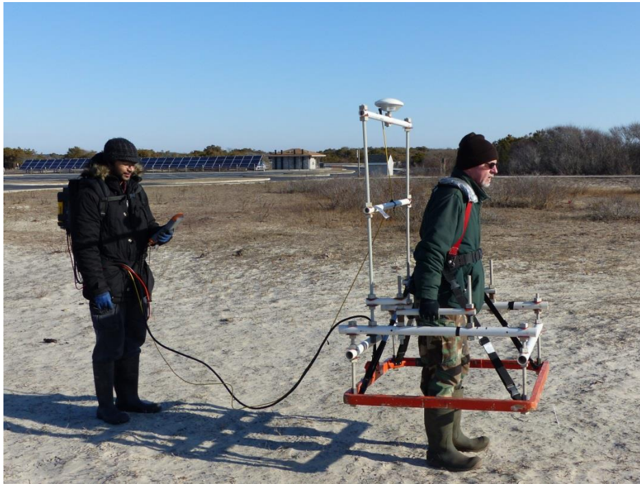
FIGURE 1-5 1x1 METER COIL CONFIGURED IN SKIRT MODE
