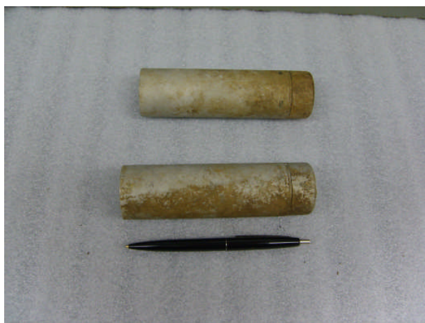
Photo E.18 – Inert MD in Prince William Forest Park museum collection-suspected 40 mm illumination rounds (side view).
