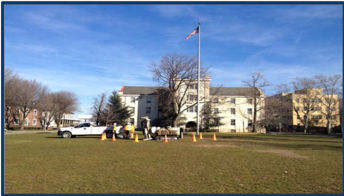
Exhibit 3: Collection of soil samples with a direct-push technology drilling rig on the former Parade Ground
