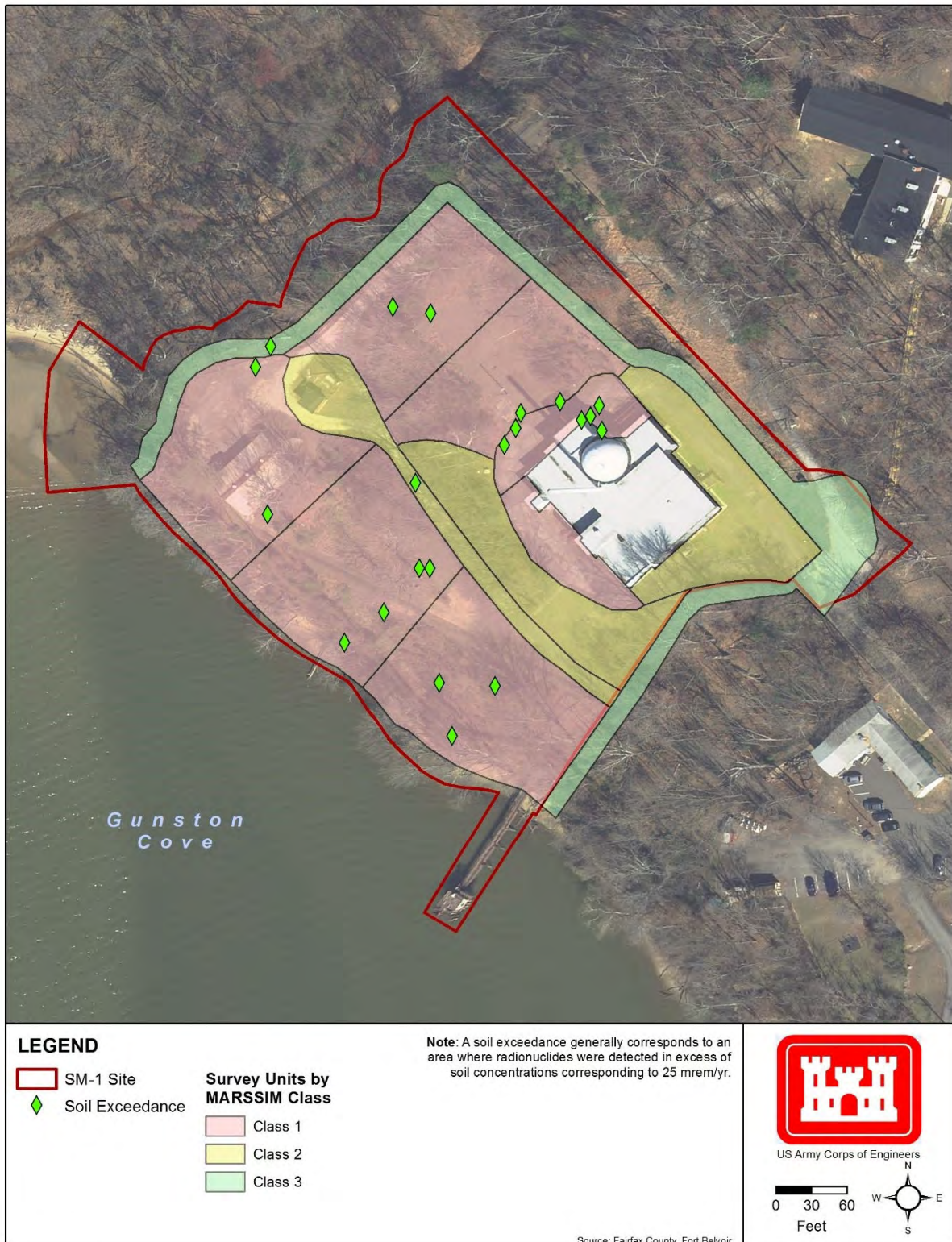
Figure 3.6-3: Contaminated Areas of Concern on SM-1 Site
