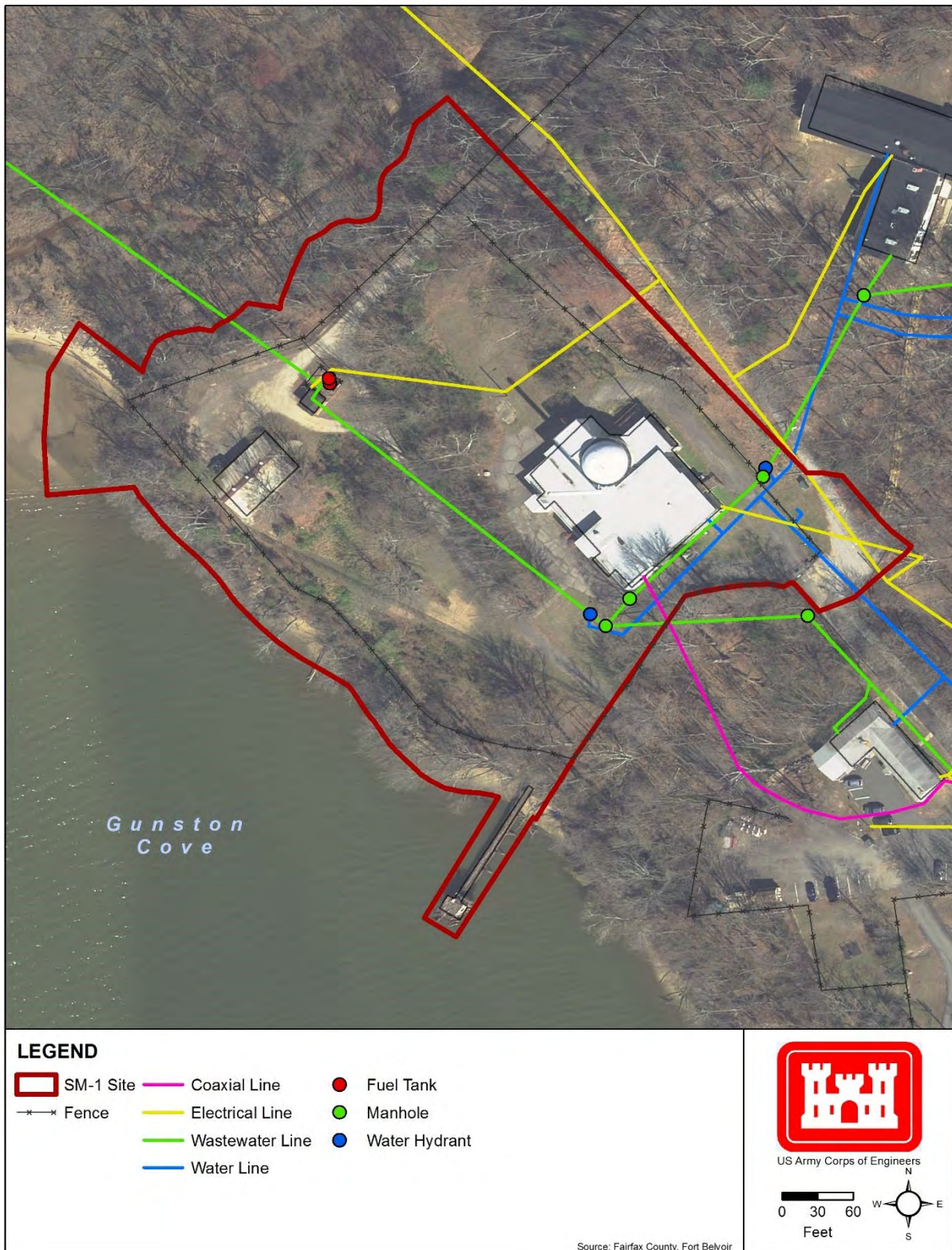
Figure 2.2-1: Existing Utilities and Infrastructure on the SM-1 Site
