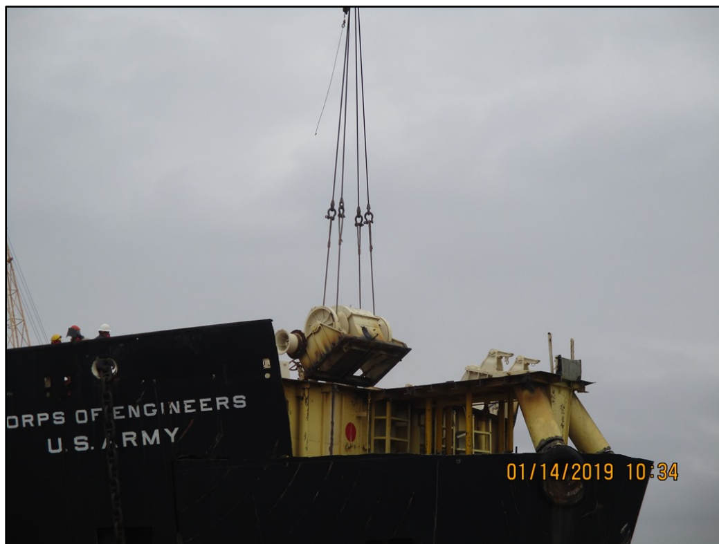
Anchor winch being removed via crane
