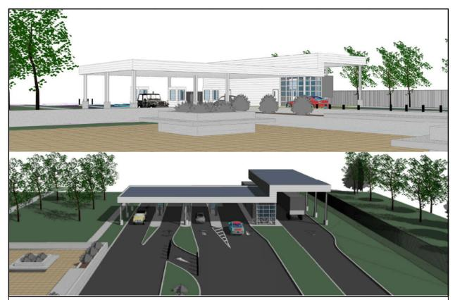
**Figure 3.3:** Proposed entrance and access control point perspective, ICC-B Development Plan, (February 2011 Concept Plan). Inset at top highlights improved traffic management principles; note the use of separate screening area for large vehicles and incorporation of grass medians to improve the aesthetics and sustainable design features of the site.
