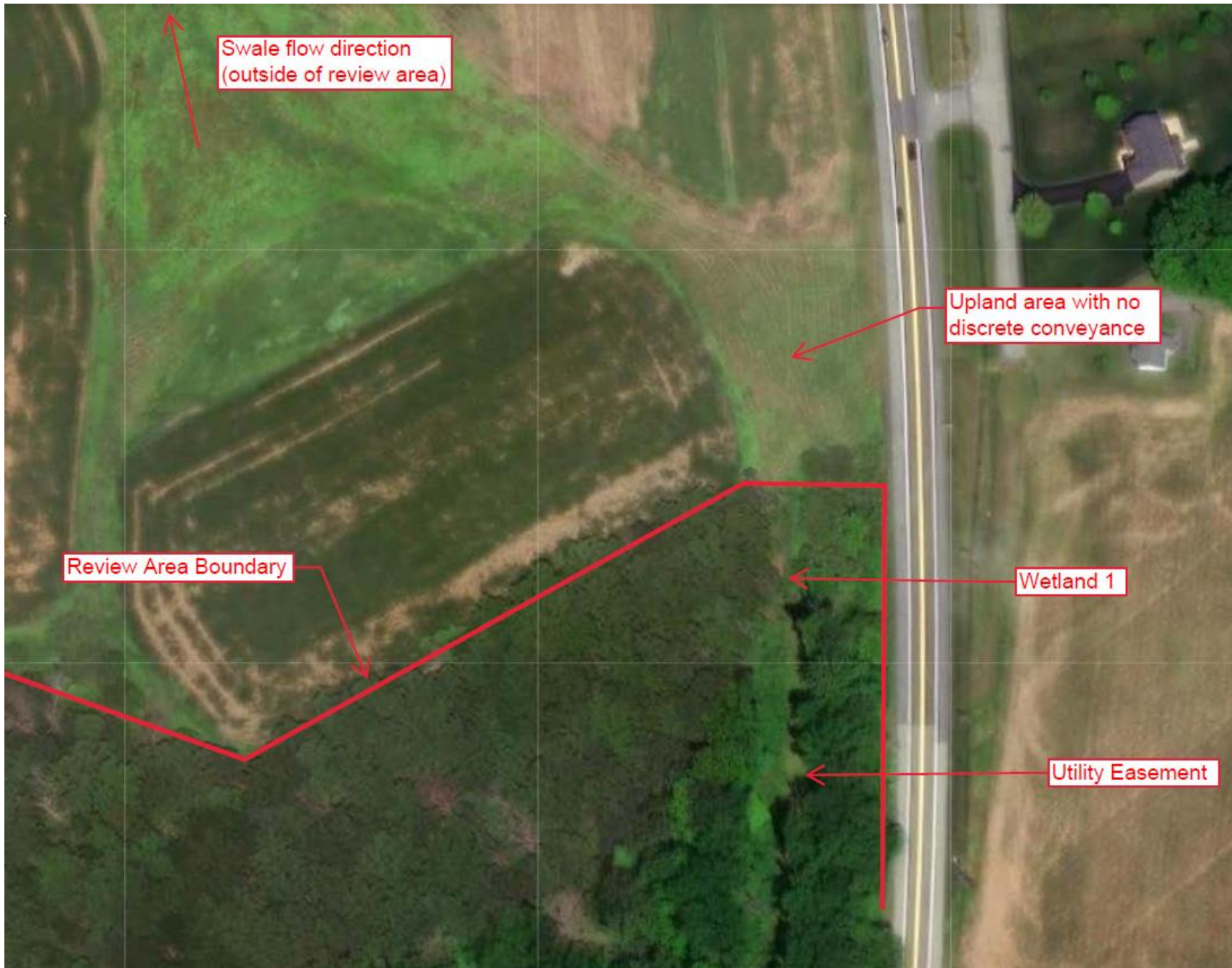
Figure 2: Aerial Imagery Showing location of Wetland W-1 in relation to agricultural swale; Accessed via the Watershed Resources Registry, March 2024.
