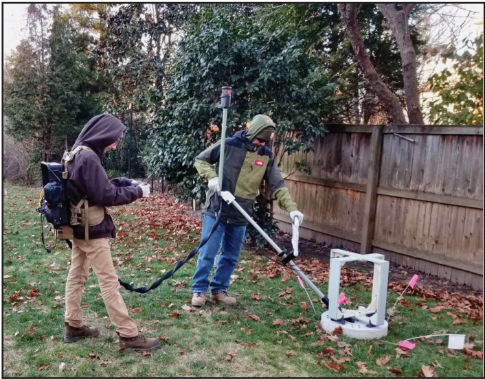
In January, contractors use the Manned Portable Vector to further examine buried metallic anomalies identified during geophysical surveys at one of the 33 residential properties that comprise the first wave of homes out of the 92 identified to be part of the Remedial Action. Of those 33 properties, nearly 14 have completed anomaly removal and have begun restoration. The MPV equipment is able to help determine whether buried metallic anomalies are munitions items or harmless cultural debris.
