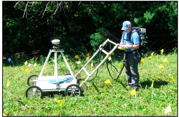
Advanced Classification technology, specifically a TEMTADS, being used to map the subsurface as part of Unexploded Ordnance Removal at New Boston Air Force Station in New Hampshire.
