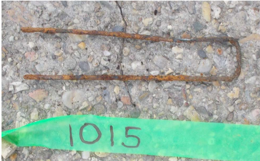
Photo 21: Target 1015, wire (lawn staple, a commonly found item), 4740 Quebec Street. Tape is 1 inch wide. MPV Fit item: MkIV booster. TEMTADS Fit item: 37 mm projectile. Date: 6 October 2016
