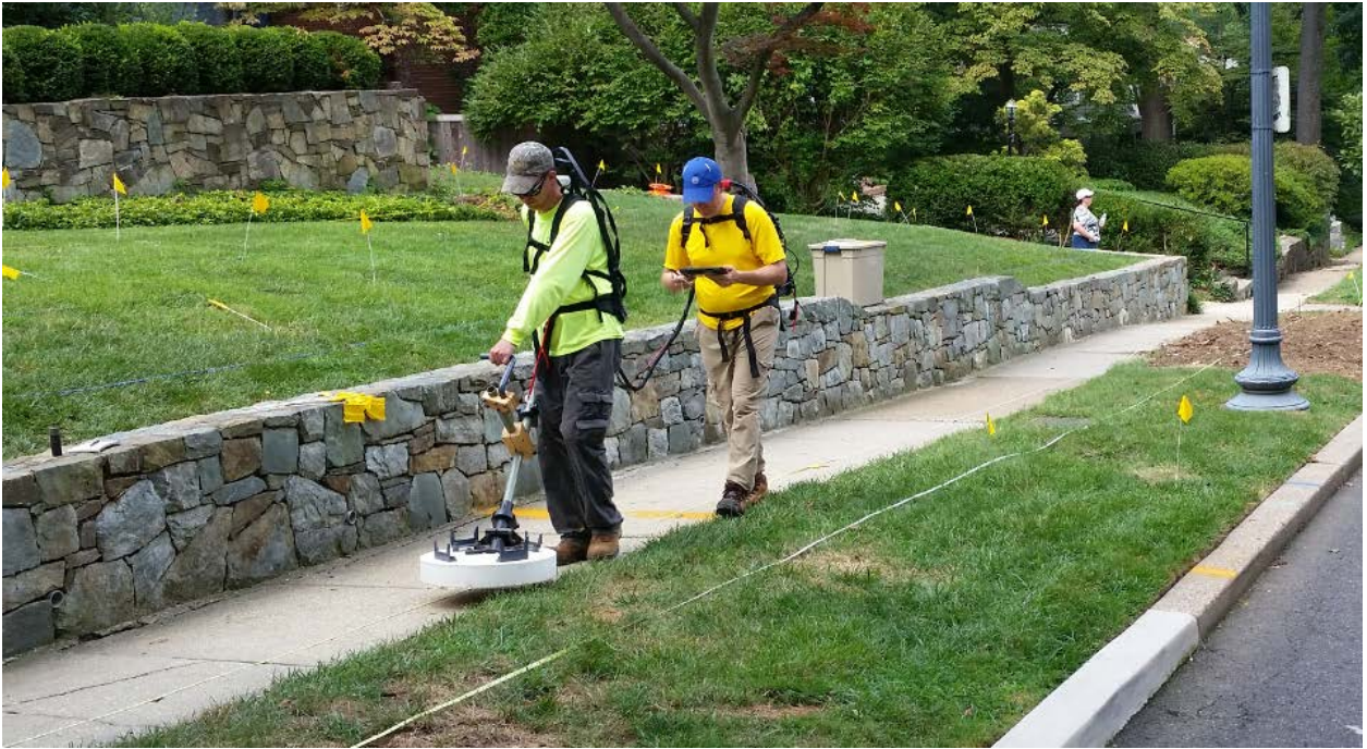
Photo 07: MPV dynamic survey with RTK GPS, 4720 Quebec Street. Date: 19 August 2016
