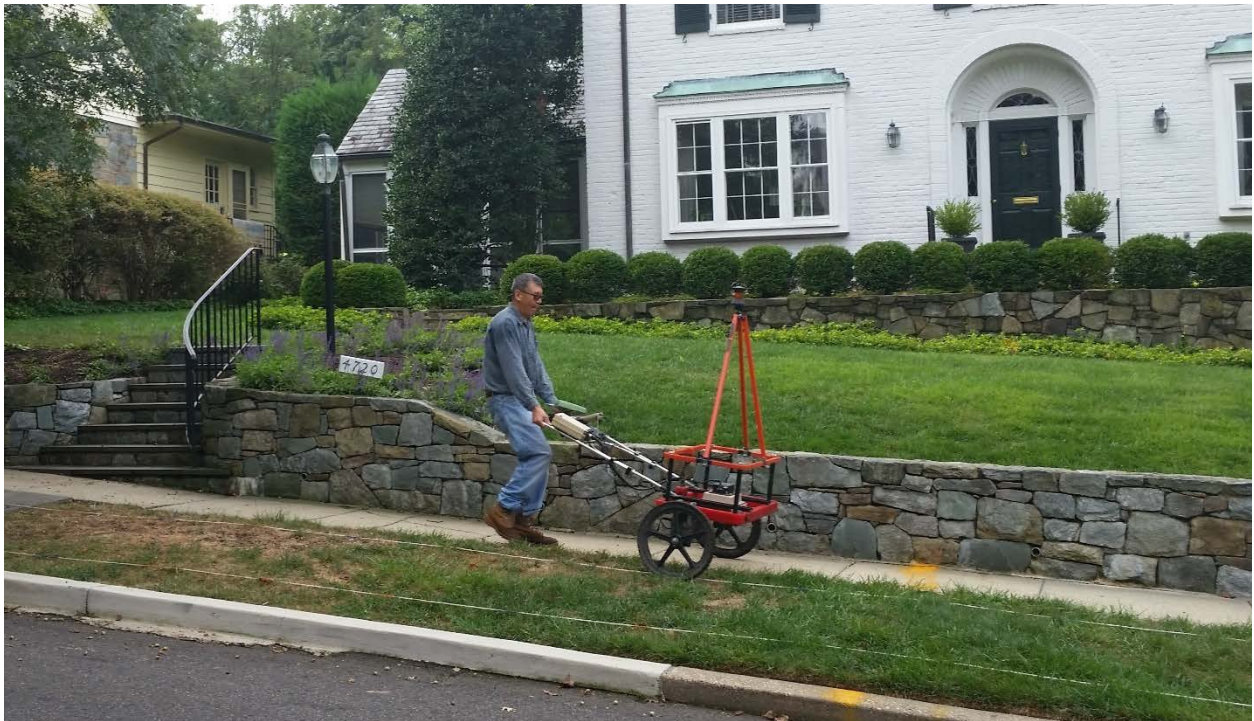
Photo 11: EM61MK2A dynamic survey with RTS, 4720 Quebec Street. Date: 20 September 2016
