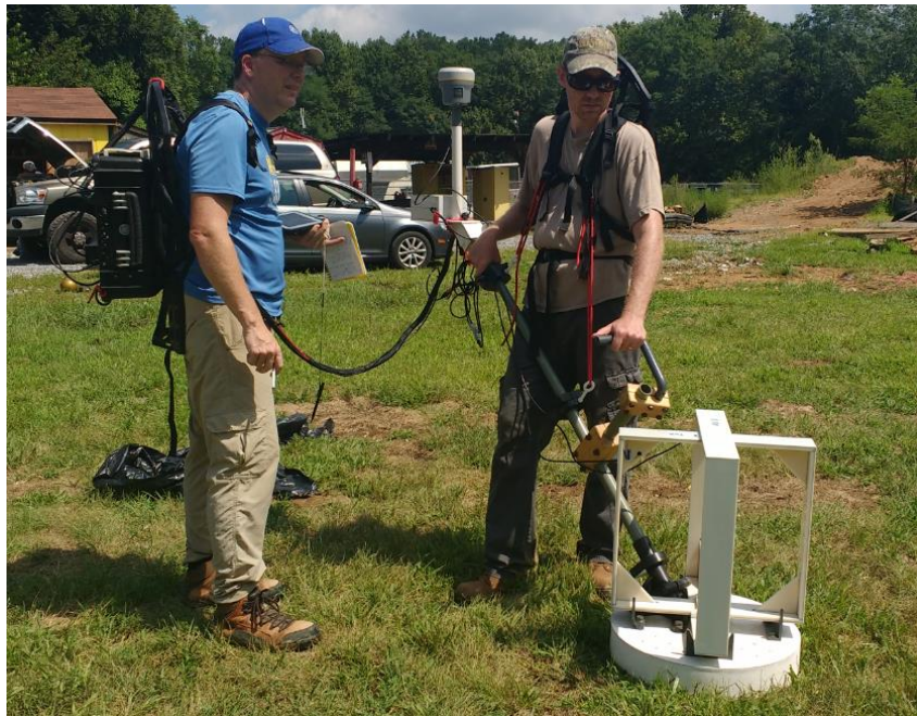
Figure 2 Cued interrogation surveying with the MPV. In cued mode, an additional two transmitter coils are added to the system for improved illumination of the buried target. The instrument is held stationary, thereby reducing sensor noise.
