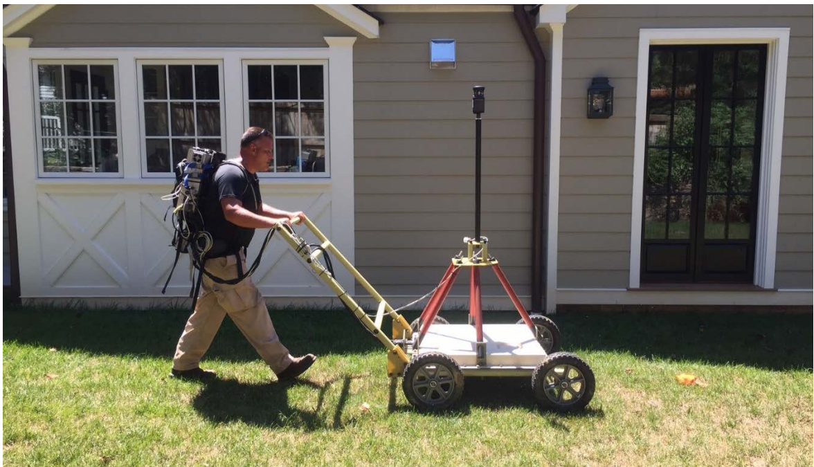
Photo 10: TEMTADS dynamic survey with RTS, 4733 Woodway Lane. Date: 16 August 2016
