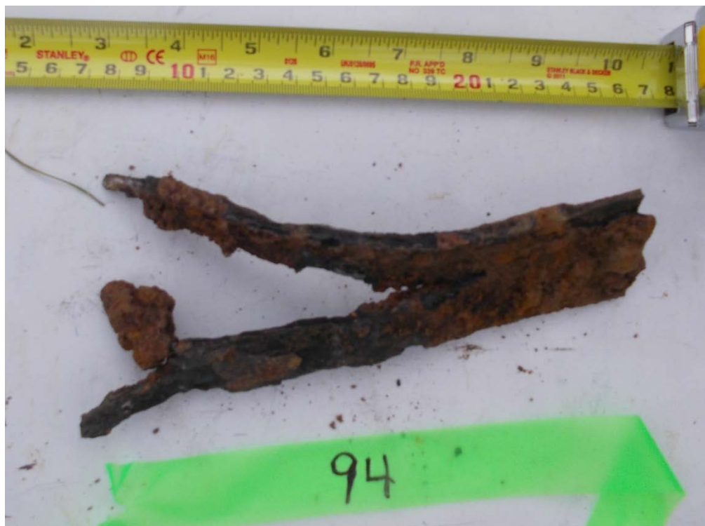
Photo 17: Target 94, munitions debris, 4720 Quebec Street. MPV Fit item: MkIV booster. TEMTADS Fit item: 37 mm projectile. Date: 14 November 2016
