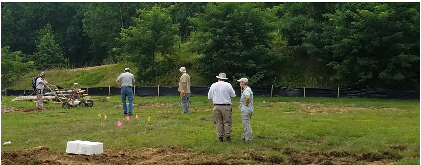
Figure 5. The TEMTADS 2x2 is at the north end of the IVS line. The pink and yellow pin flags in the foreground define the IVS static background location.
