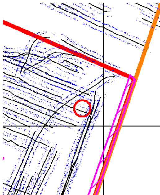
Figure 1 – Tracklines for the TEMTADS 2x2 in the vicinity of Blind Seed #16. Black solid lines indicate the course over ground of the sensor array. The blue dots indicate the located positions of the individual sensors. The red circle is the location of Blind Seed #16.
