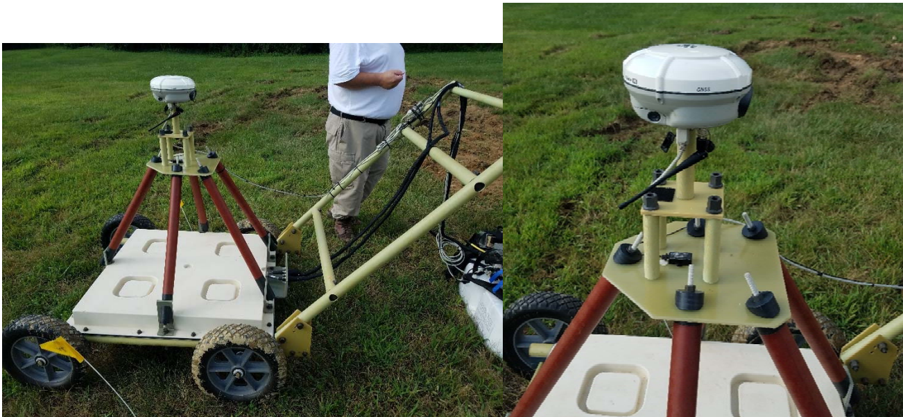
Figure 1. TEMTADS sensor after assembly with RTK GPS. The figure on the right shows the orientation of the IMU sensor.
