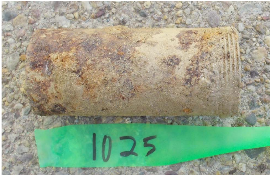
Photo 22: Target 1025, pipe, 4740 Quebec Street. Tape is 1 inch wide. MPV Fit item: MkIV booster. TEMTADS Fit item: Small ISO. Date: 5 October 2016
