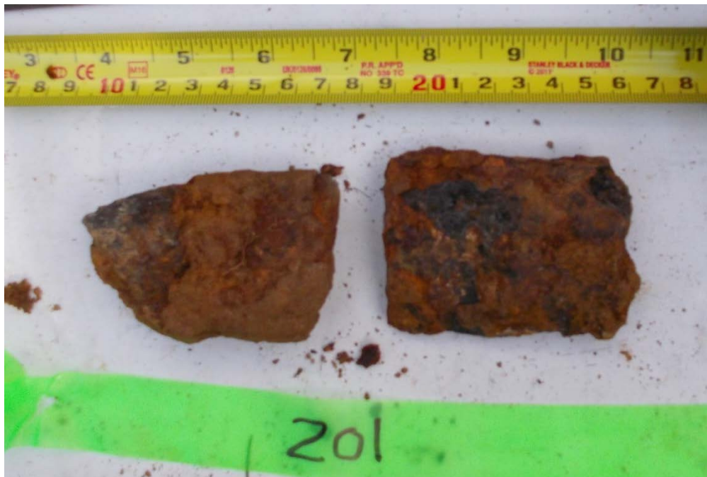
Photo 19: Target 201, munitions debris, 4720 Quebec Street. MPV Fit item: Stokes Mortar. TEMTADS Fit item: 37 mm projectile. Date: 15 November 2016
