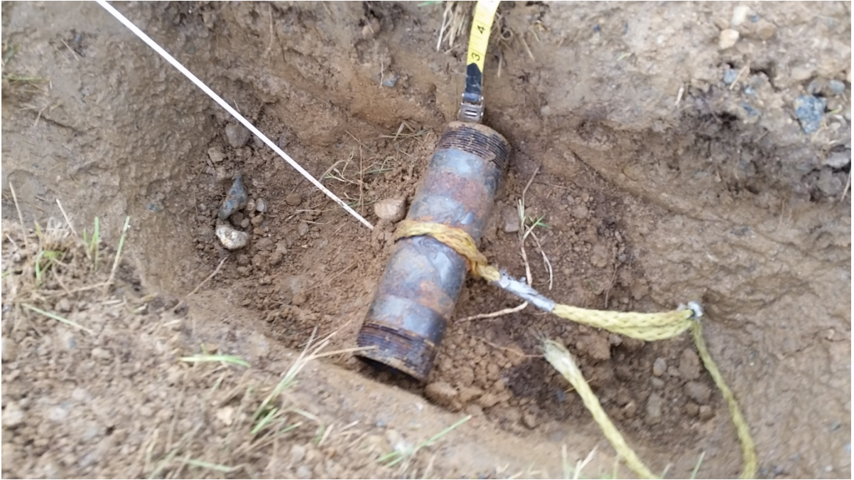
Photo 03: IVS-3, Medium Industry Standard Object (2 inch diameter pipe nipple)
