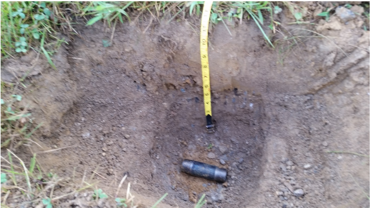
Photo 04: IVS-4, Small Industry Standard Object (1 inch diameter pipe nipple)
