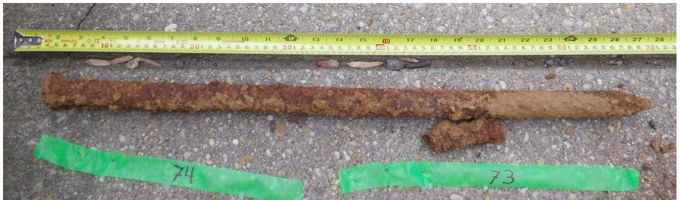
Photo 16: Target 73/74, steel spike, 4720 Quebec Street. MPV Fit item: MkIV booster/75 mm. TEMTADS Fit item: 37 mm projectile/3 inch projectile. Date: 14 November 2016
