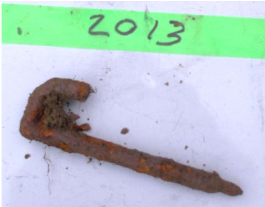
Photo 24: Target 2013, tent stake, 4733 Woodway Lane. Tape is 1 inch wide. MPV Fit item: Small ISO Schedule 80. TEMTADS Fit item: 37 mm projectile. Date: 5 October 2016
