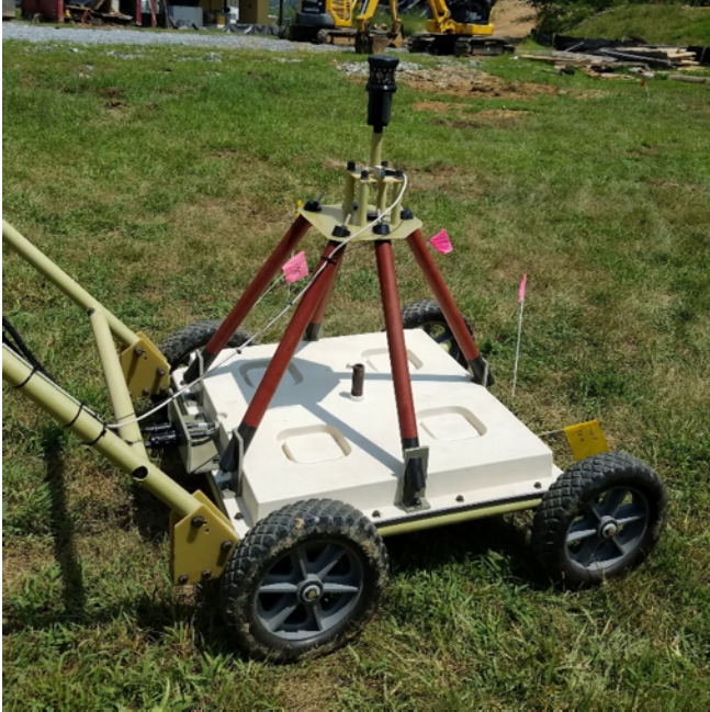
Figure 2. TEMTADS sensor after assembly with RTS prism.
