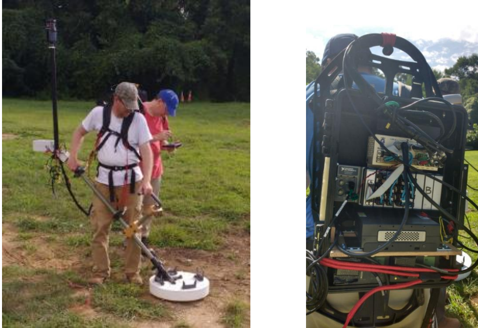
Figure 1 The MPV electromagnetic induction metal detector. Left: MPV surveying in dynamic mode, using RTS for positioning. Right: Photo of electronics, data acquisition system, and computer mounted on field backpack.
