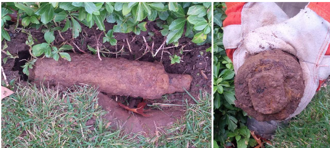
Photo 18: Target 129, Stokes Mortar, unfuzed, 4720 Quebec Street. MPV Fit item: Stokes Mortar. TEMTADS Fit item: 5 inch projectile. Date: 14 November 2016
