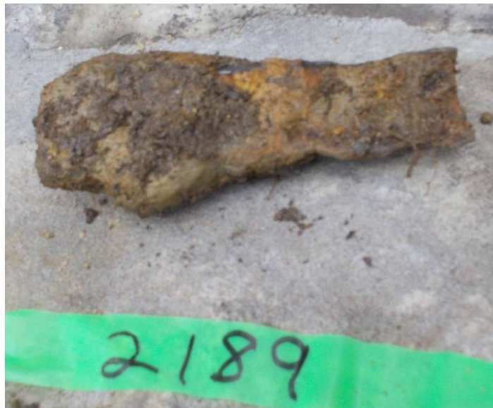
Photo 26: Target 2189, steel scrap, 4733 Woodway Lane. Tape is 1 inch wide.
