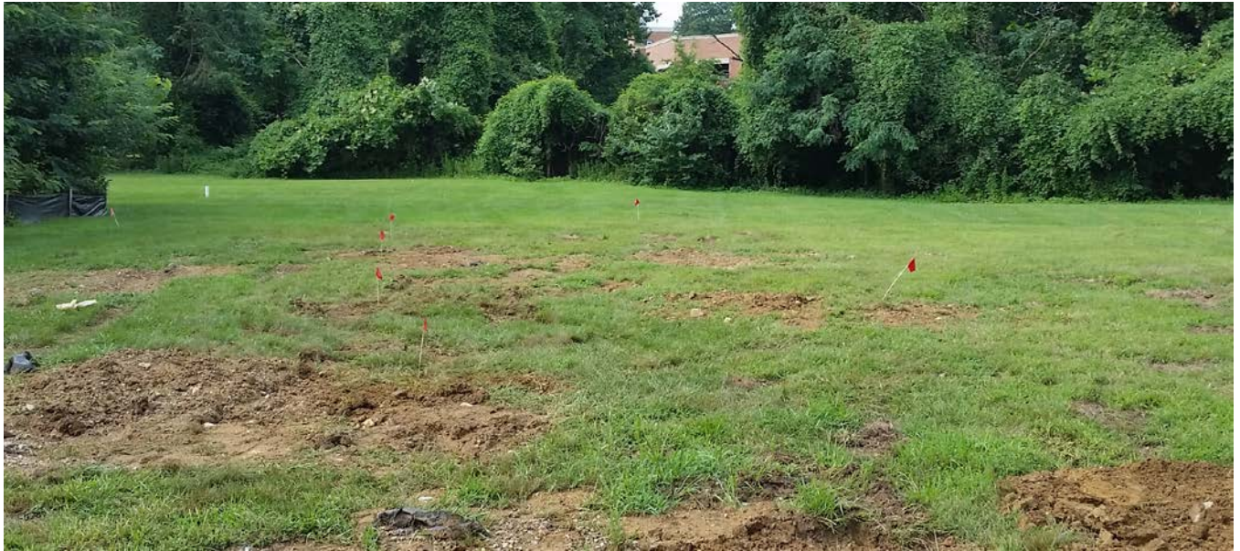
Photo 05: Completed IVS. Four flags at left indicate seed line and two flags at right indicate noise line.
