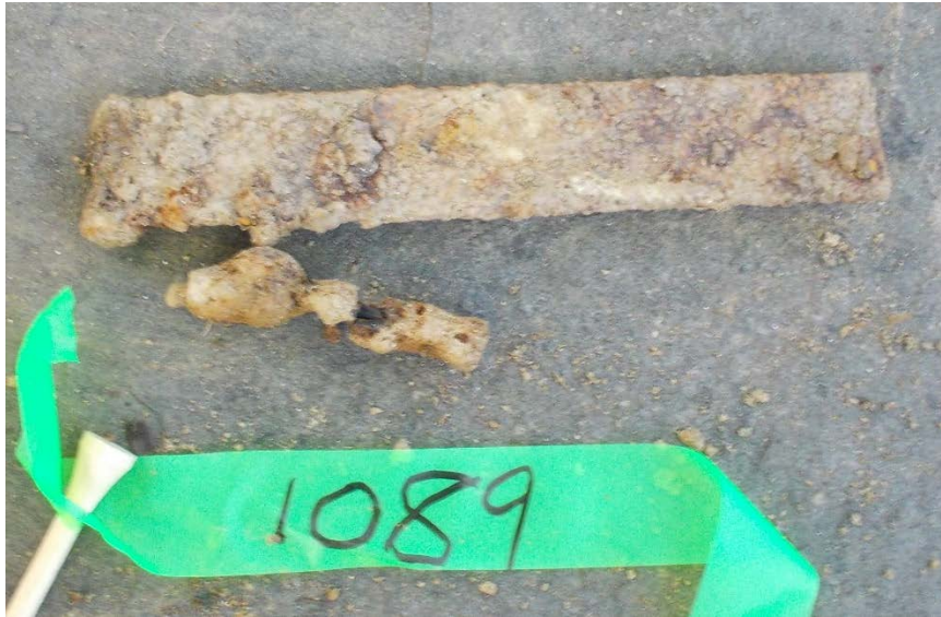
Photo 23: Target 1089, steel band, 4740 Quebec Street. Tape is 1 inch wide. MPV Fit item: Stokes Mortar. TEMTADS Fit item: none. Date: 5 October 2016
