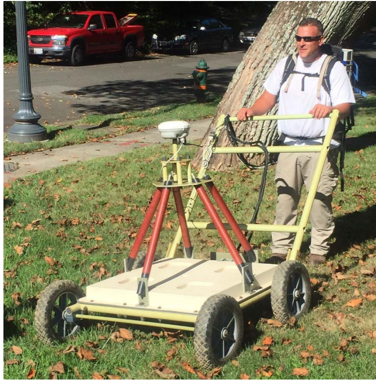
Photo 09: TEMTADS dynamic survey with RTK GPS, 4733 Woodway Lane. Date: 15 August 2016
