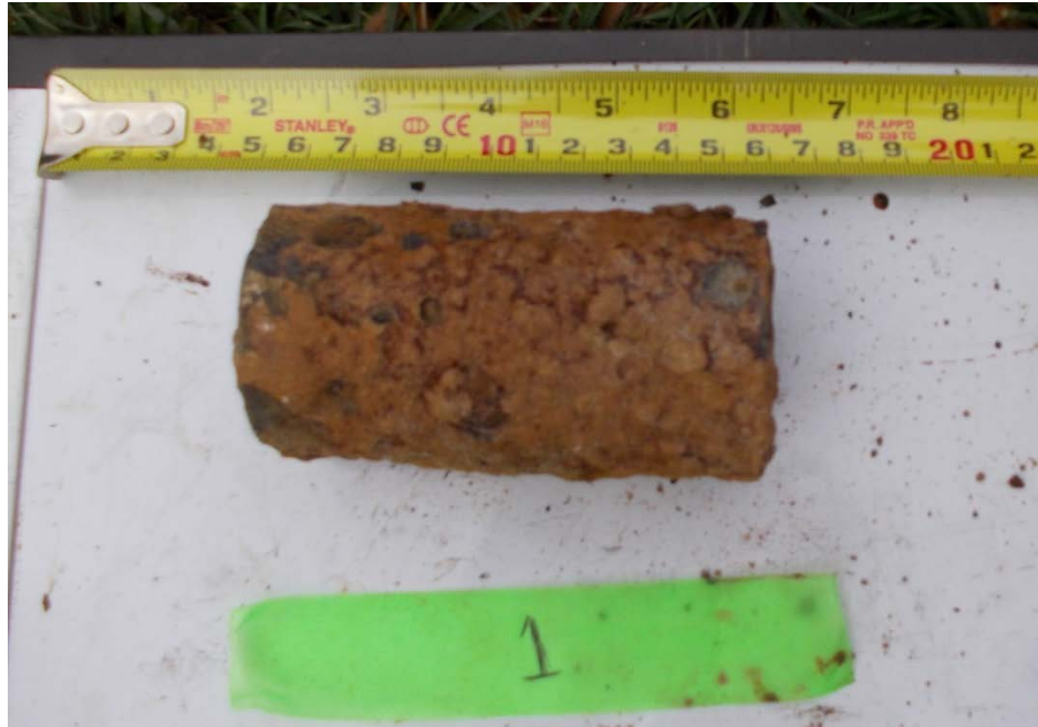
Photo 15: Target 1, pipe fragment, 4720 Quebec Street. MPV Fit item: MkIV booster. TEMTADS Fit item: Small ISO. Date: 15 November 2016
