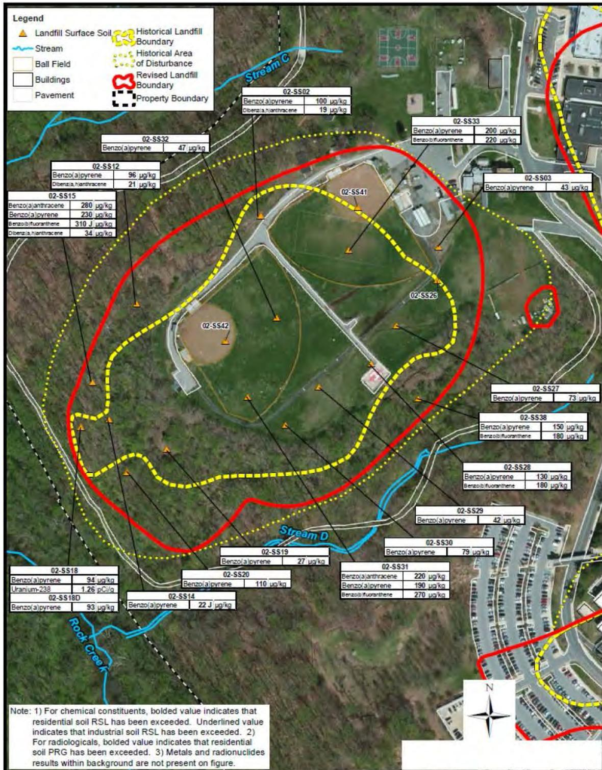
Figure 4-4: Significant sampling results in surface soils
