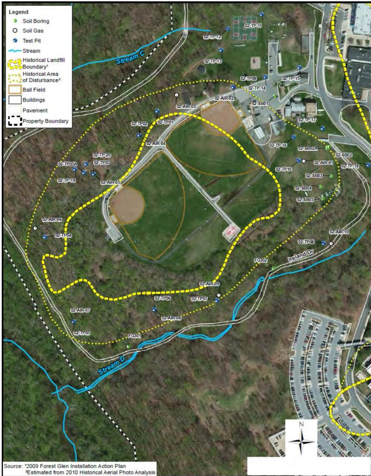
Figure 4-5: Subsurface soil sample locations
