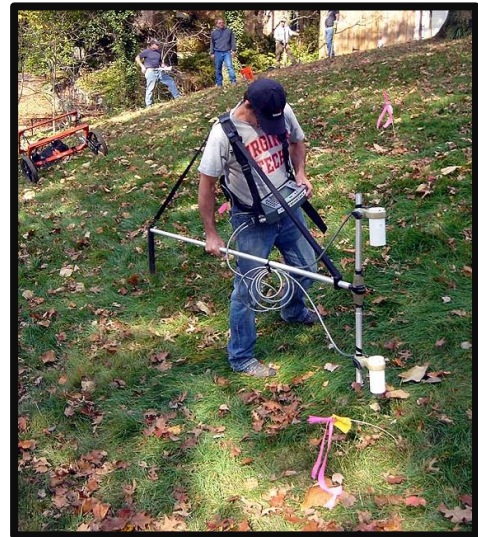
Reacquiring Exact Anomaly Location with the Geophysical Instrument G858
