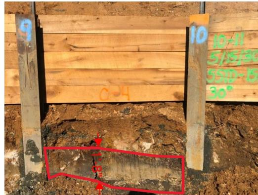
Sidewall at Piles 9 & 10. Dark AUES layer at wall, 1 ft 8 in thick
