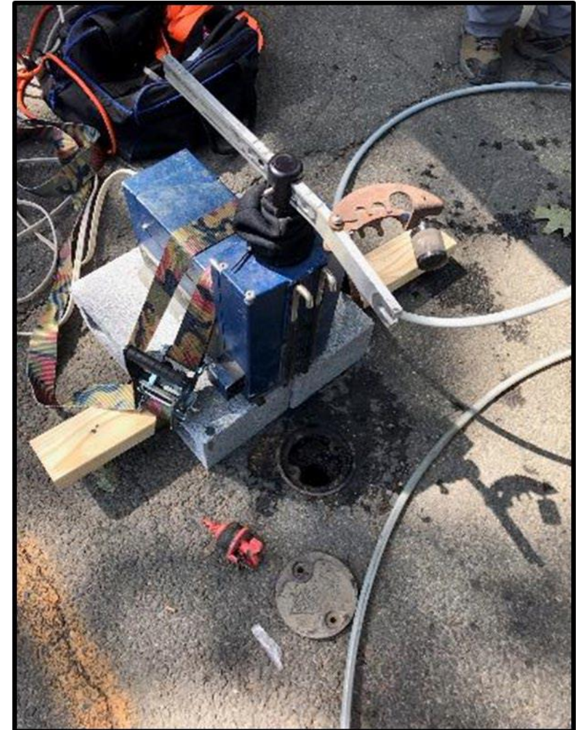
Groundwater sampling well
