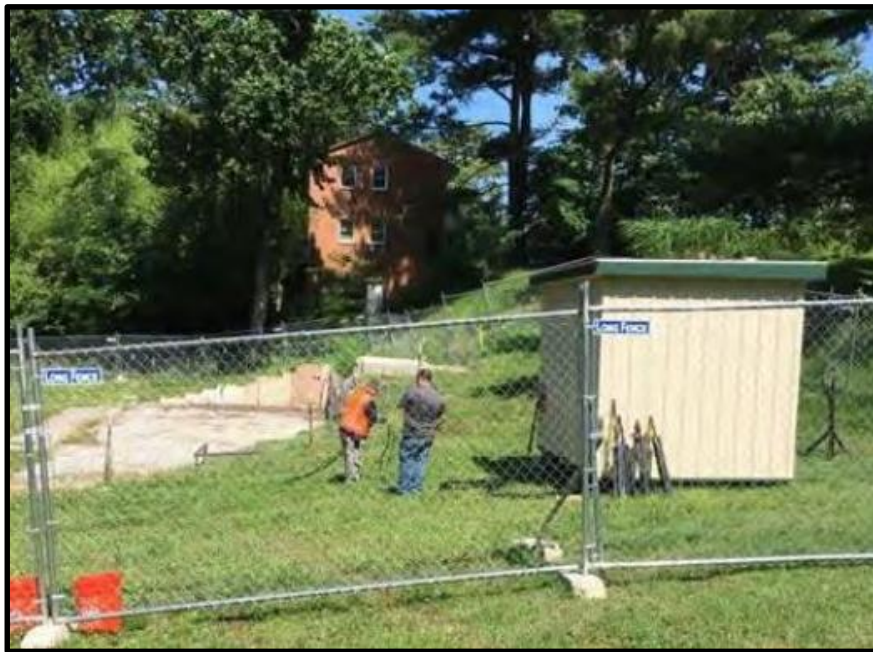
MINICAMS Shed present for air monitoring at the former PSB during sub-slab soil sampling
