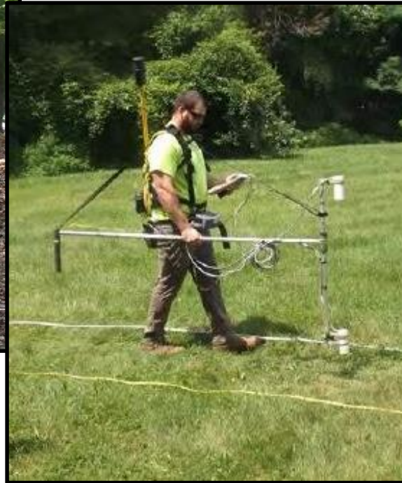
Geophysicists conducting test survey with magnetometer (G-858) at the Federal Property
