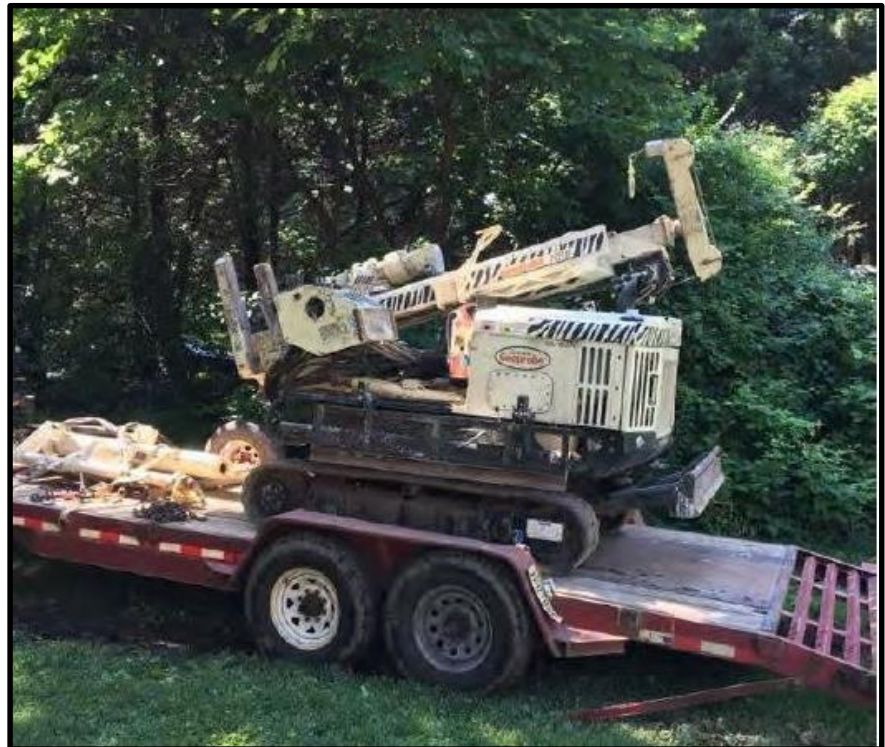
Geoprobe for subsurface soil sampling
