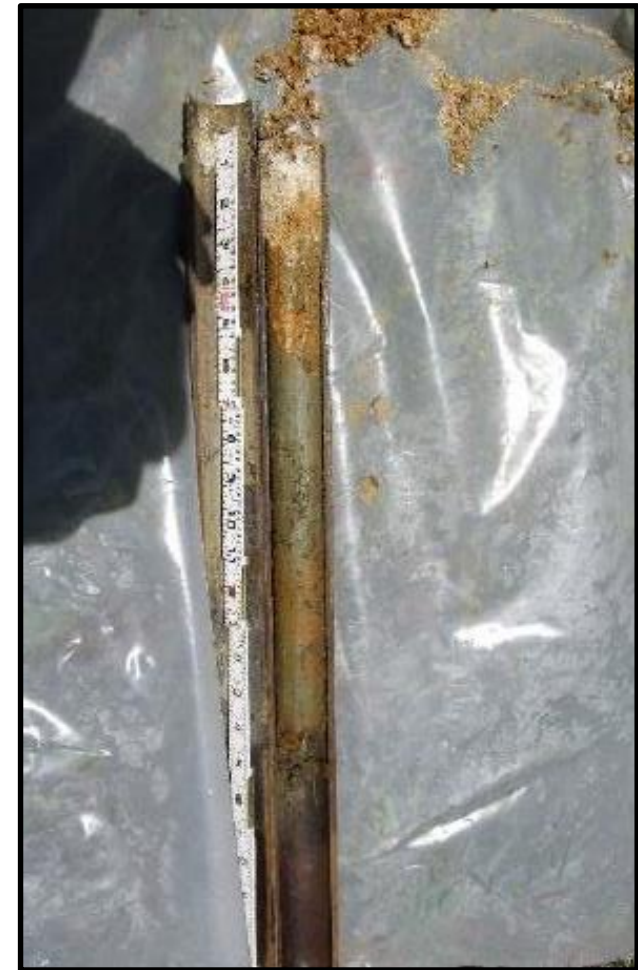
Typical soil core in split spoon collection from boring
