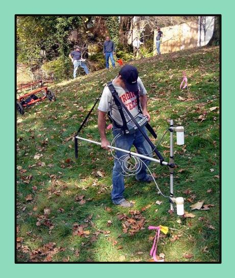
Reacquiring exact anomaly location with the G-858 Magnetometer
