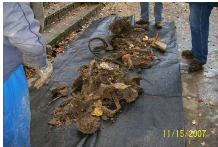
Cultural debris consisting primarily of construction debris with bricks, metal, insulation, wire, terracotta pipe, pulley, wire rope, soda bottle fragments, chicken wire, and porcelain, was recovered from depths between 4 and 12 ft bgs.
