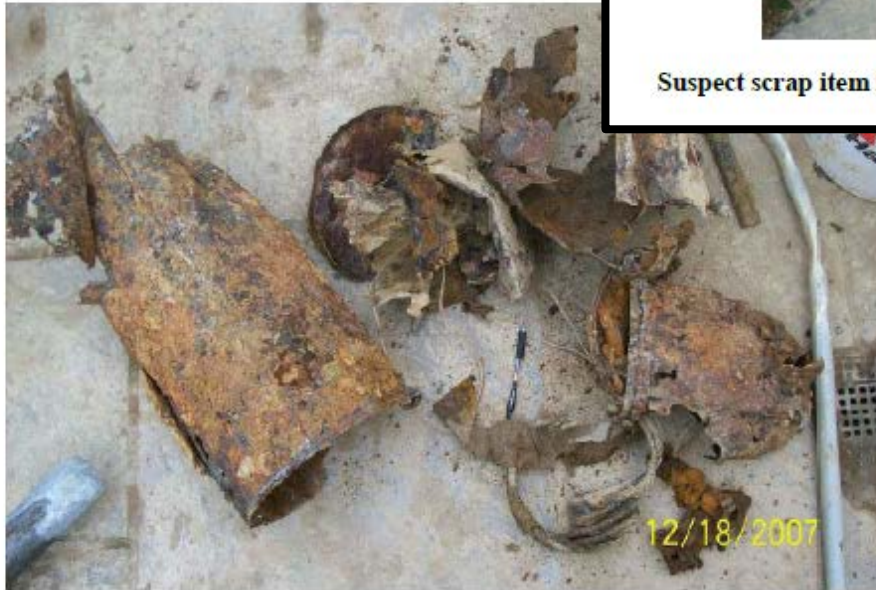
Cultural debris consisting of PVC tubing, metal pipe, and metal debris present from 0 to 1 ft bgs and from 4 to 5 ft bgs.
