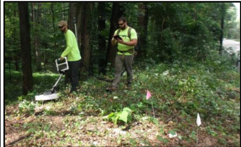
Geophysicists conducting dynamic survey with magnetometer (G-858) in Dalecarlia Woods
