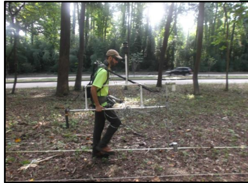
Geophysicists conducting dynamic survey with magnetometer (G-858) in Dalecarlia Woods
