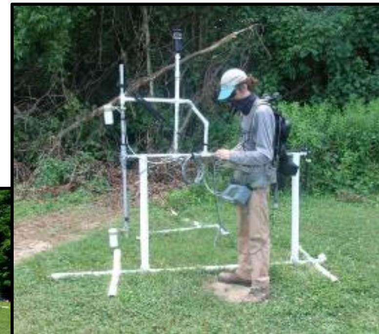
Function tests with the G-858 magnetometer
