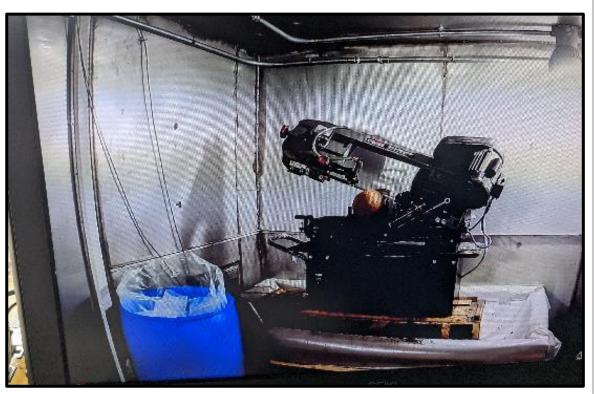
A remotely operated saw cutting munitions debris item
