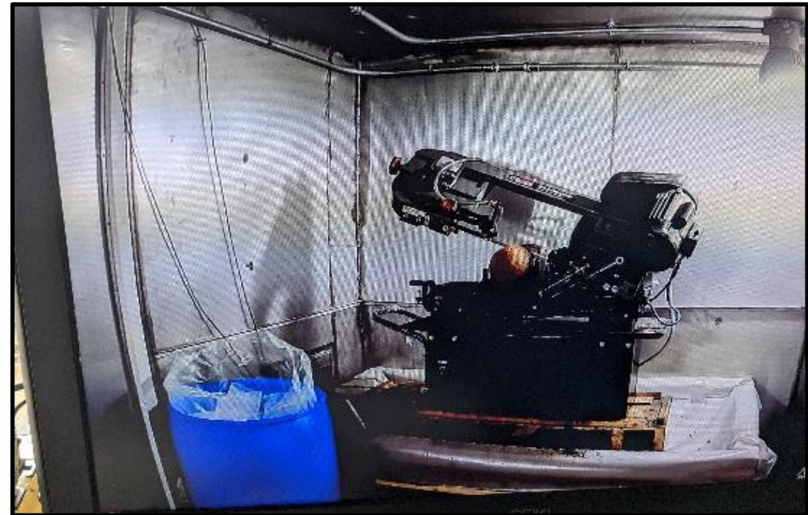
*A remotely operated saw cutting munitions debris item*
