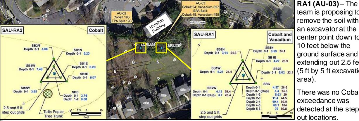
team is proposing to remove the soil with an excavator at the center point down to 10 feet below the ground surface and extending out 2.5 feet (5 ft by 5 ft excavation area).
