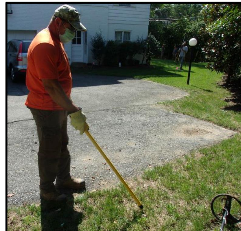
***The team uses analog metal detector to detect anomaly before digging***
