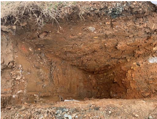
Test Pit E8 excavated to 7 ft. bgs
