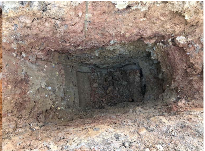
Test Pit E7 excavated to 6 ft. bgs
