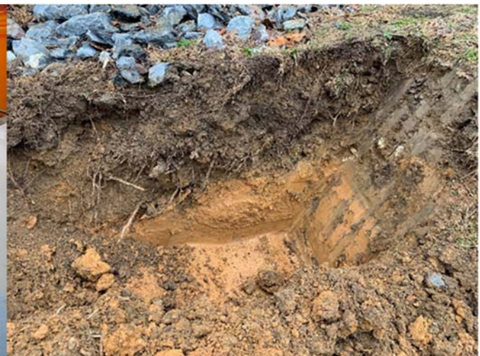
Test Pit E2F2. Note transition from impacted material (top)
