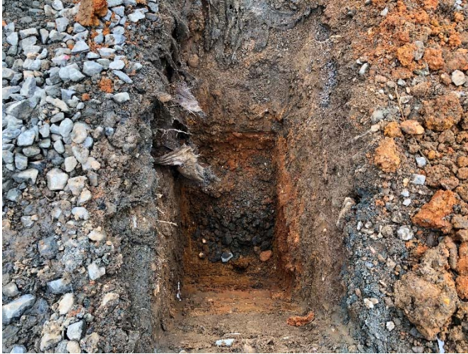
Test Pit F7G7 excavated to 5 ft. bgs
