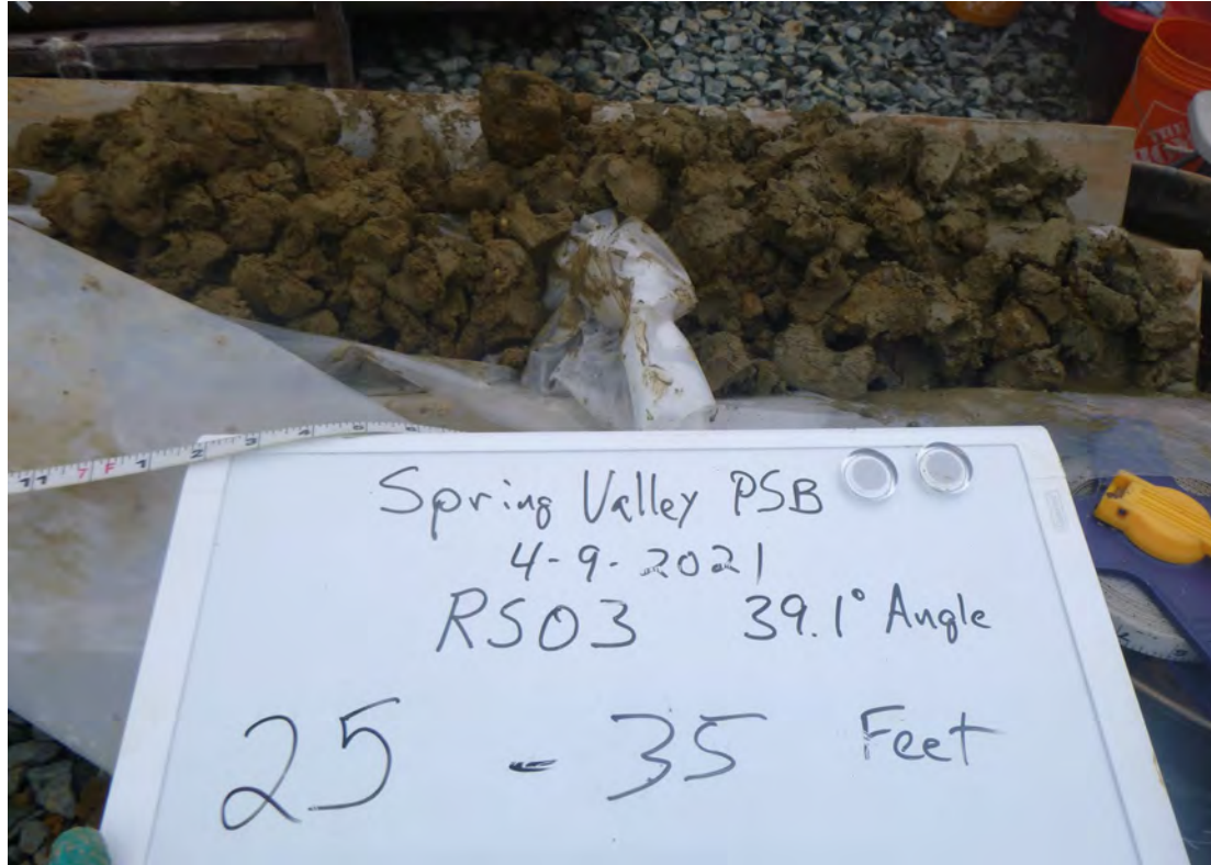
Rotosonic borehole RS-03 soil core on table after UXO Techs checked and sorted any debris and Geologist described the soil properties.
