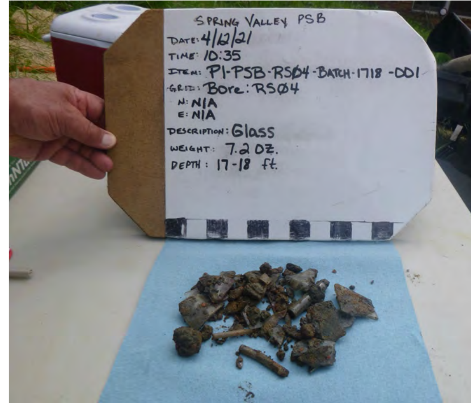
Rotosonic borehole RS-04 glass debris encountered at 17-18 feet with sample collected for CCDC headspace screening.
