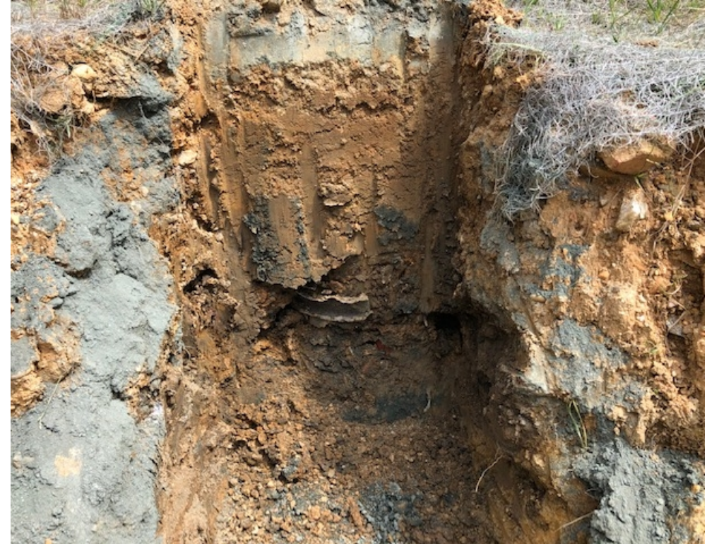
North Wall Grid D3 – Test pit into the North Sidewall – chasing the dark AUES debris layer @ 6 feet from slab.
