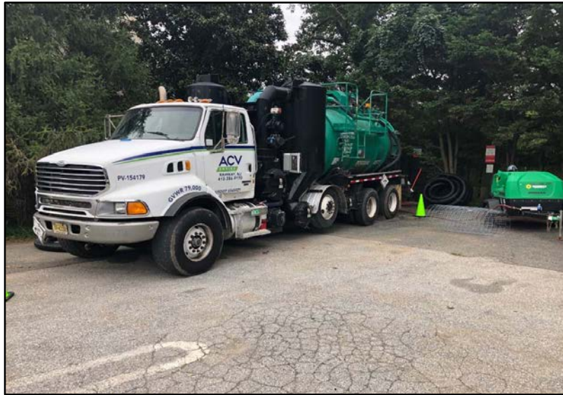
Soil vacuum truck and air compressor used for air-knife operations.
