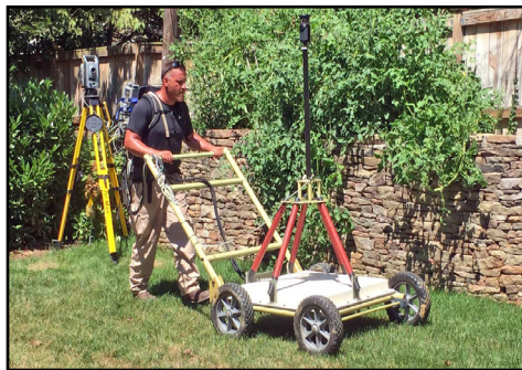
One of the Advanced Classification technologies being used to map the subsurface of a property in Spring Valley as part of ongoing Pilot Project field work.
