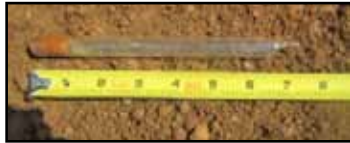
Sealed test tube of crystallized CN (tear gas, not a chemical agent) (May 21, 2013)
